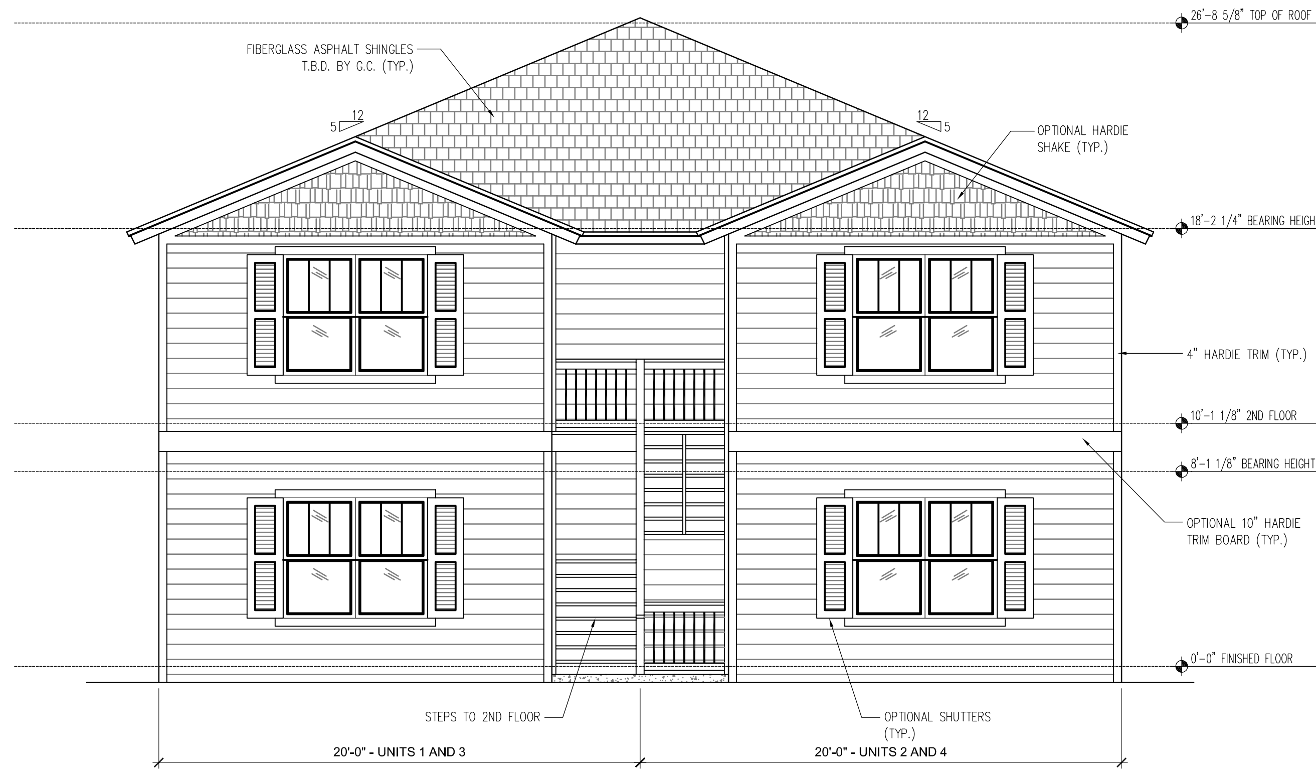
2 FRONT ELEVATION "B" - DOUBLE GABLE A5 1/4" = 1'-0"
